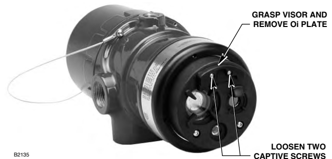
Figure 17—Oi Plate Removal
